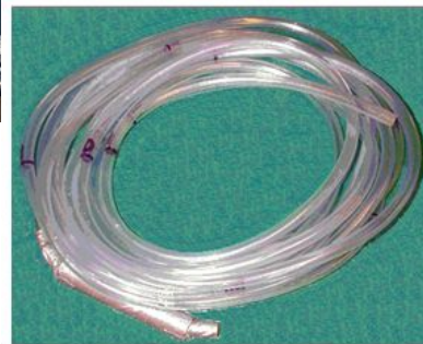
Weighted core tubing for collecting phytoplankton and chlorophyll
